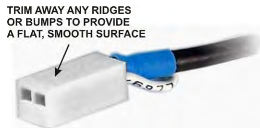
Figure 54. Preparing the KXV3B TMP Cable for Installation.
