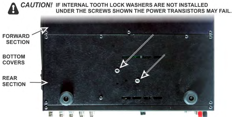
Figure 101. Checking Power Transistor Mounting Hardware.
