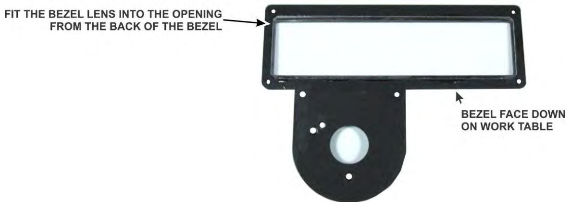
Figure 15. Fitting the Bezel lens in the Bezel.
