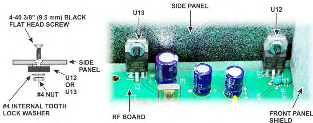
Figure 75. Attaching U12 and U13 to the Right Side Panel.
