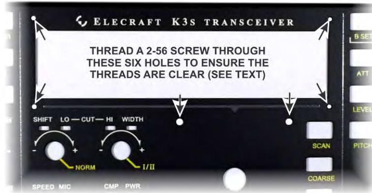
Figure 10. Checking Front Panel 2-56 Threaded Screw Holes.
