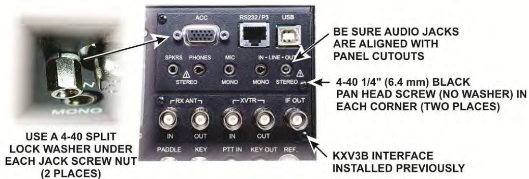
Figure 61. Mounting the KIO3B Connector Panel.
