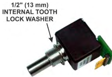
Figure 12. VFO A Encoder Assembly Preparation for Installation.
