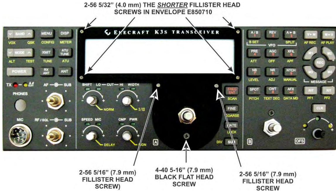
Figure 16. Mounting the Bezel.
