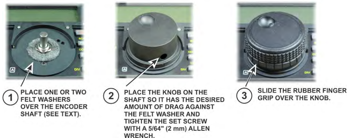
Figure 20. Mounting the VFO A Tuning Knob.
