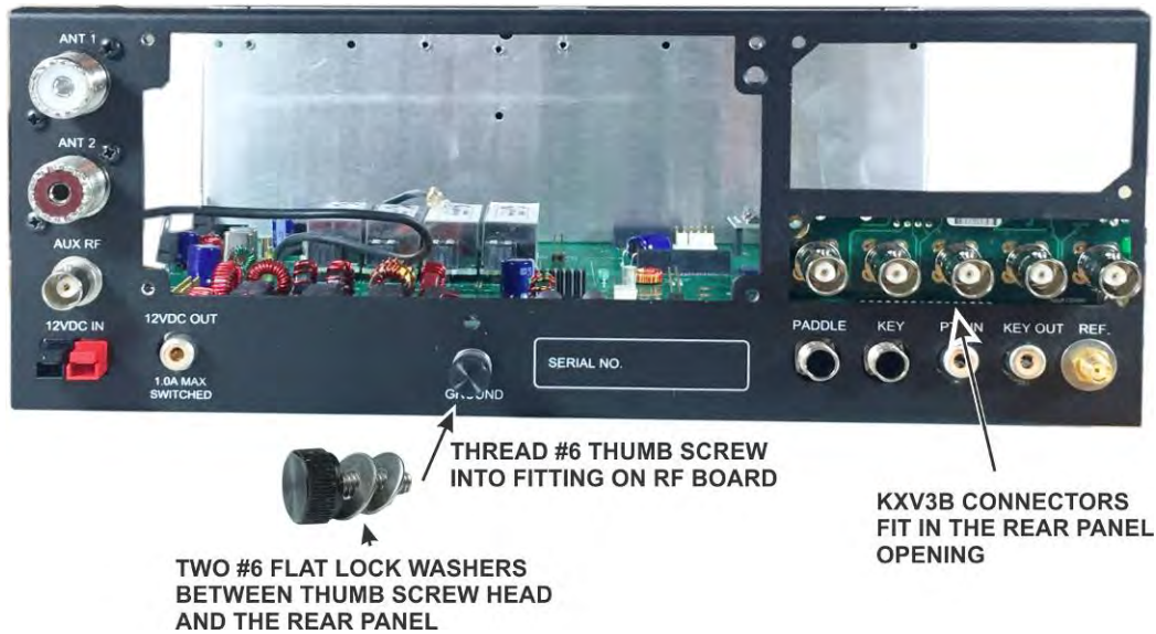
Figure 49. Mounting the Rear Panel.
