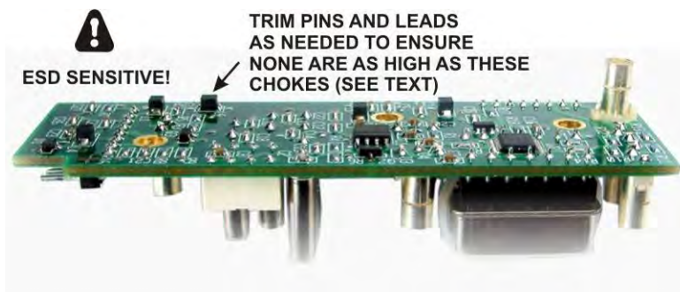
Figure 79. Checking Lead Lengths on KREF3 Board.
