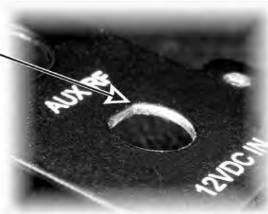
Figure 45. Removing the Powder Coating from the AUX RF Connector Hole.
