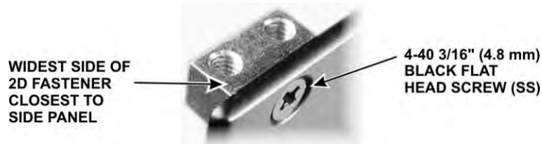
Figure 65. Installing Left Side Panel 2D Fastener.
