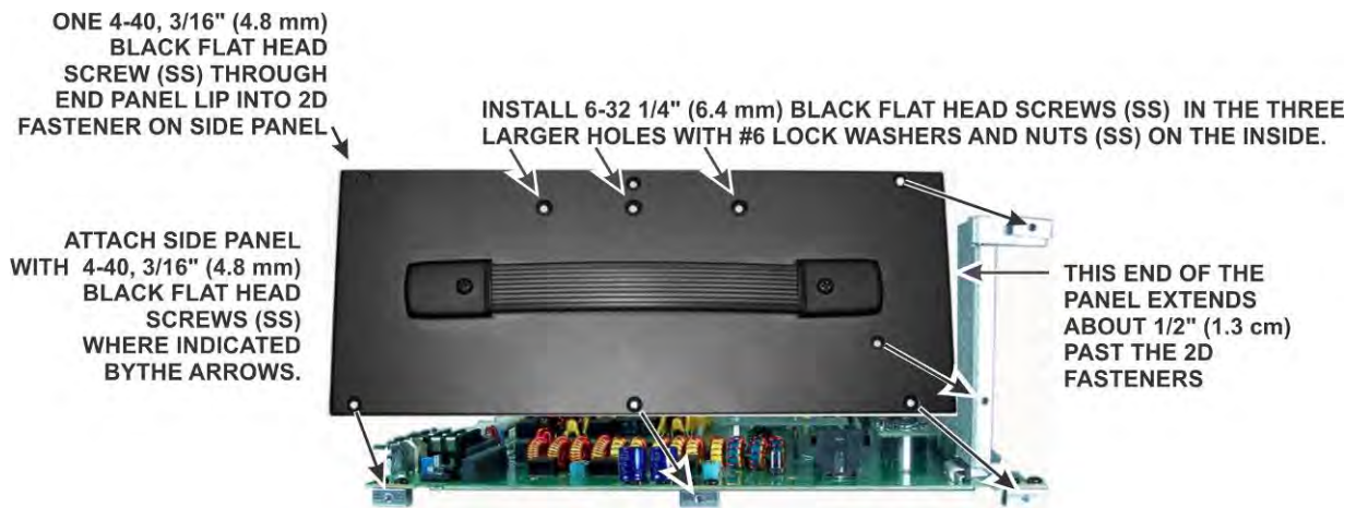
Figure 66. Mounting Left Side Panel.
