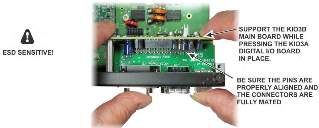
Figure 60. Installing the KIO3A Digital I/O Board.
