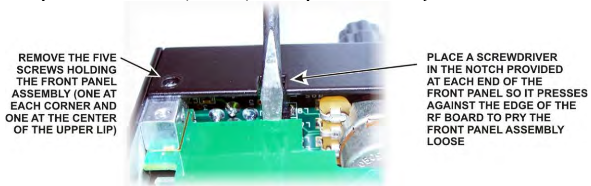
Figure 53. Removing the Front Panel.
